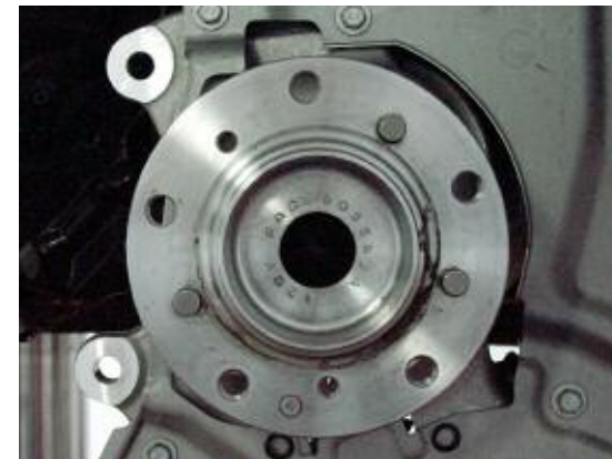
Detail of Rotor Alignment Pins on Hub
